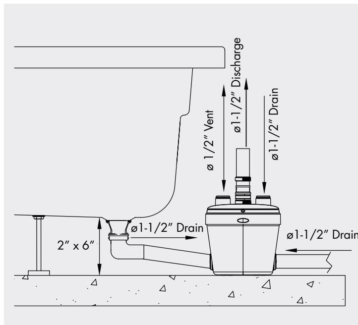
AN EASY SOLUTION FOR A REMOTE LAUNDRY ROOM INSTALLATION OR FOR ANY GRAY WATER APPLICATION
